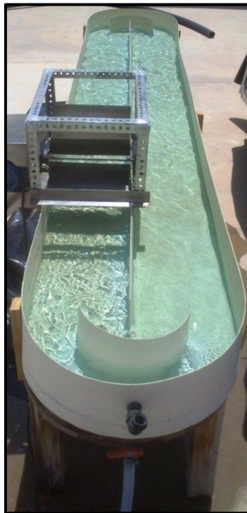
Figure 2.6. 360-L Raceway Pond Reactor.
